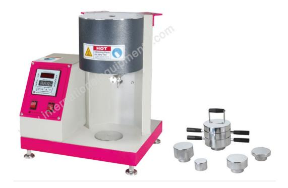
As per ASTM D 1238 & ISO 1133 - (Test Method A) to check the melt flow rate (MFR) of thermoplastics and compounds with auto cutting of flowing extrudate and prelogic facility.
